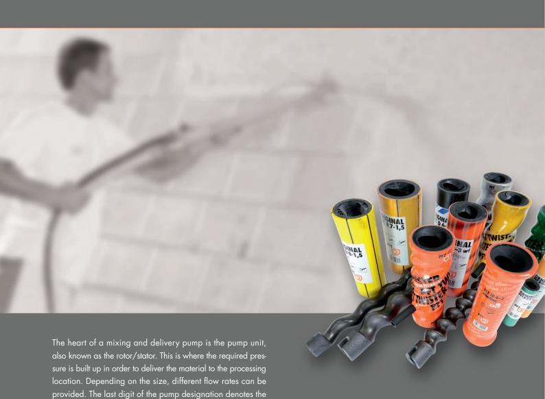
number of pressure stages; a working pressure of 10 bar can be built up for each stage. If these values are no longer achieved, the unit is worn out and should be replaced.
